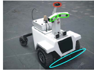
Fig. 3. Robot system. The robot is equipped with a GPS system (red), two stereo heads (green) and a bumper (cyan).
