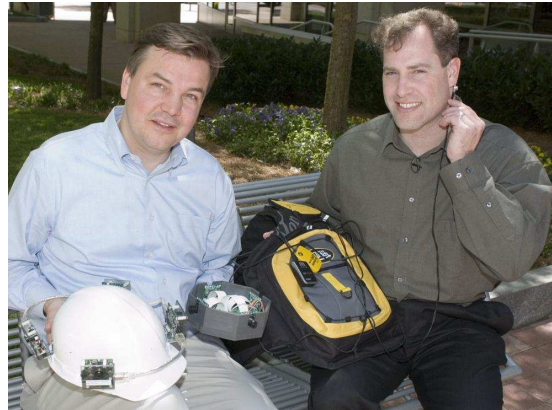
Figure 5: Prototype SWAN system. The helmet is equipped with multiple camera rig and the system aids users through auditory interface.
